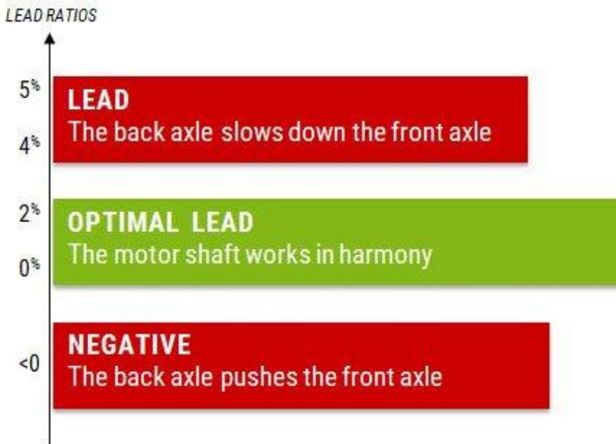
For a 4 wheel drive tractor with different diameter wheels, the right lead between front and back wheels must be obtained.
