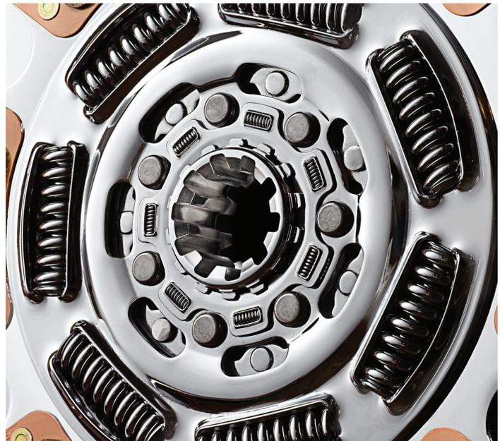
In the late 90’s, engine makers opened the flywheel bore from 8.5 inches to 10 inches. This gave clutch designers valuable extra real estate to dampen vibration produced by new engines. Eaton capitalized on this with the introduction of 7-Spring and VCT models. The damper springs in these models grew larger and heavier to provide more travel. The result is even greater ability to dampen torsional vibrations.
