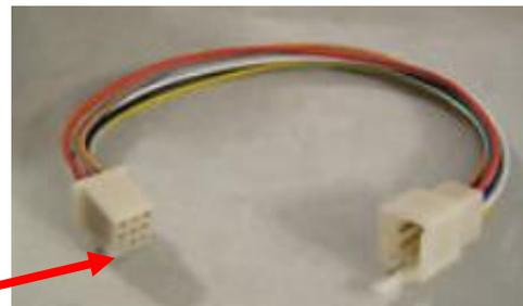
I purchased an interface harness from eBay for \$8. Adjusted the wiring pin out to line up with the Kubota colours as best as possible. Removed the 2 unused wires.
