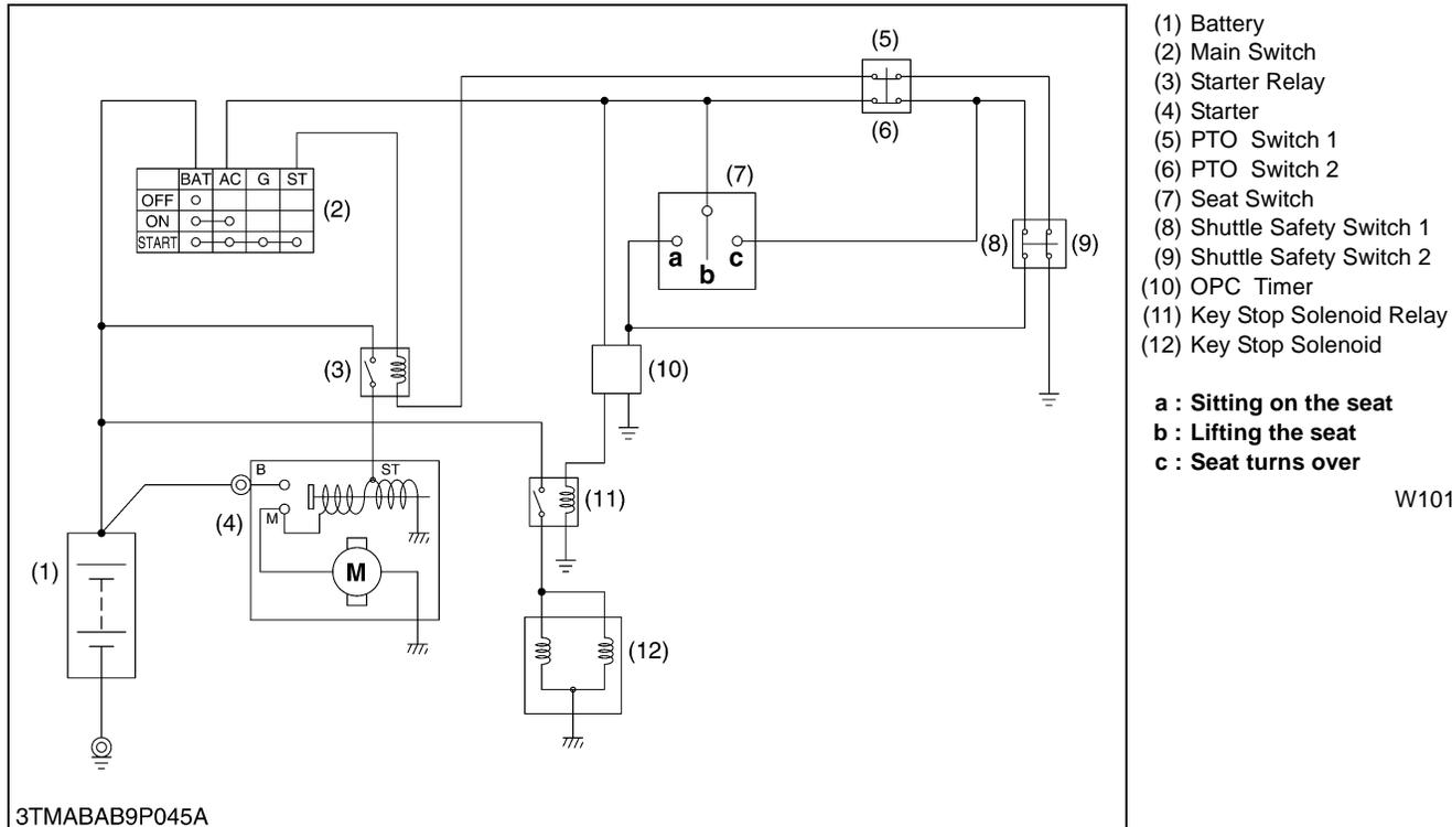
The operator presence control (OPC) system which automatically stops the engine when operator stands from the seat while shifting the PTO lever or shuttle shift lever. This system is controlled by the seat switch (7), PTO switches (5), (6), shuttle shift lever switches (8), (9), OPC timer (10), key stop solenoid relay (11), key stop solenoid (12).
