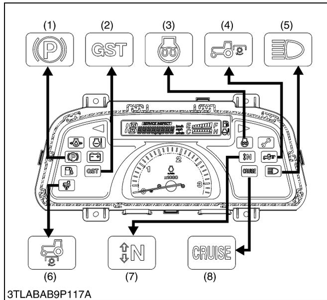
In this electronic instrument panel, the control of various monitor lamps shown in figure are equipped in addition to warning lamps.
