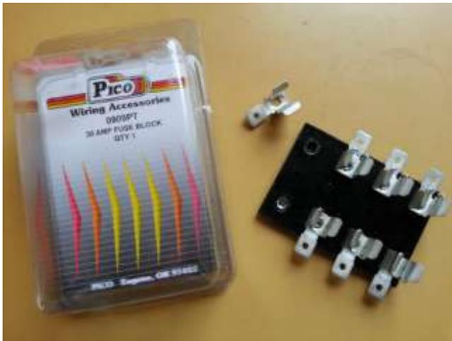
2. I used wire snips to remove the blade connectors and filed down any sharp edges.
