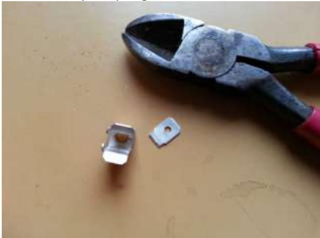
3. I then inserted the screws from the original Kubota fuse panel. I had to pry apart the barrel connectors to get the screws in, but they're soft aluminum so they bend back without effecting how the fuses clip in.
