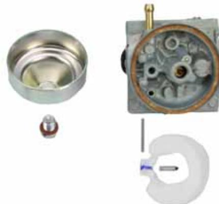
3. Remove the main jet and the main nozzle.
