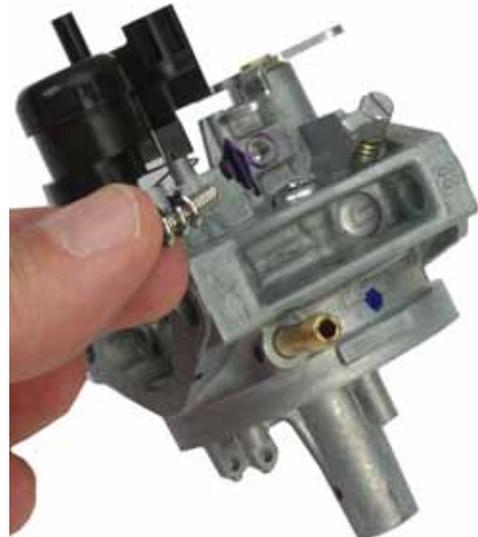
5. Remove the 5 x 6 mm screw covering the pilot jet.
