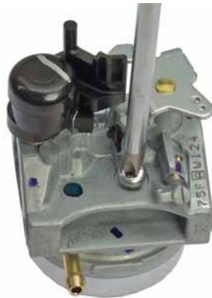
15. Check the slow speed air/pilot screw channels for obstructions.
