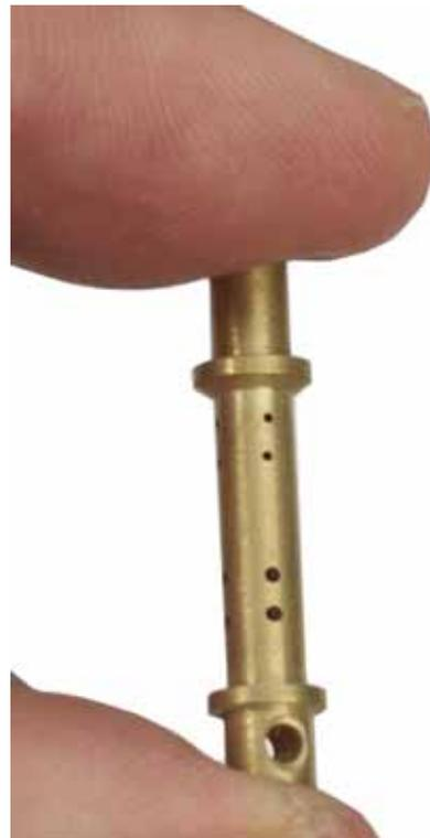
8. Clean the main jet by spraying carburetor cleaner through the jet and using the appropriate size jet cleaning tool and compressed air. Do not use a welding tip cleaning needle.
