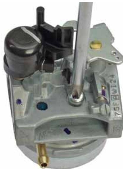
6. Clean the float valve seat using carburetor cleaner and compressed air.
