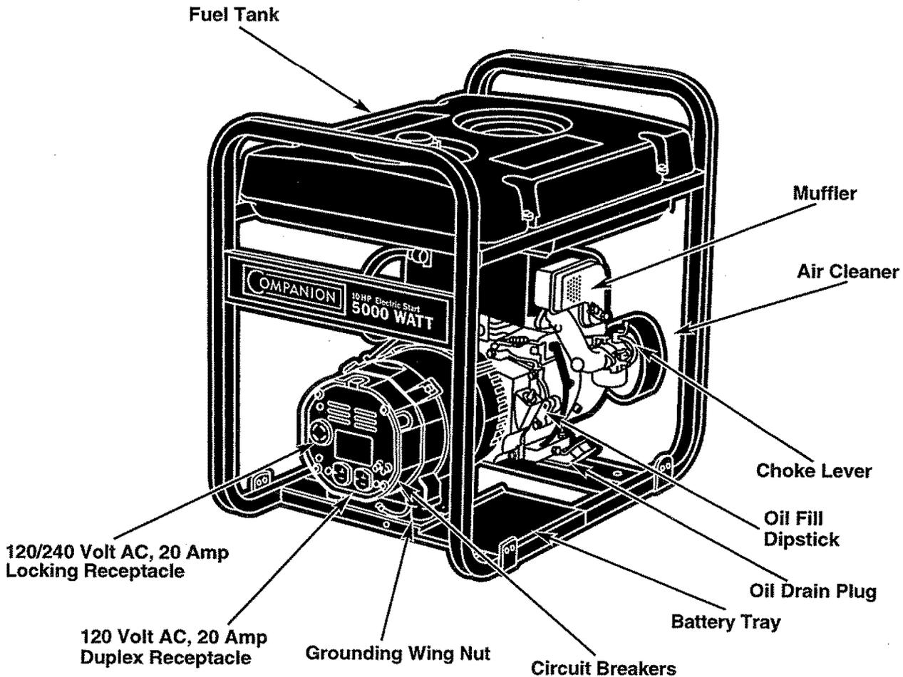
**120 Volt AC, 20 Amp, Duplex Receptacles** — May be used to supply electrical power for the operation of 120 Volt AC, 20 Amp, single phase, 60 Hz electrical lighting, appliance, tool and motor loads.
