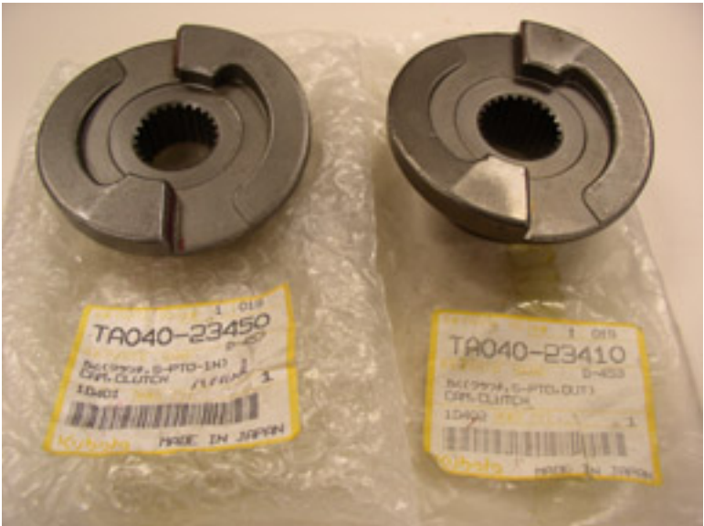
Old Style Clutch Cams (P/N TC220-99980)
