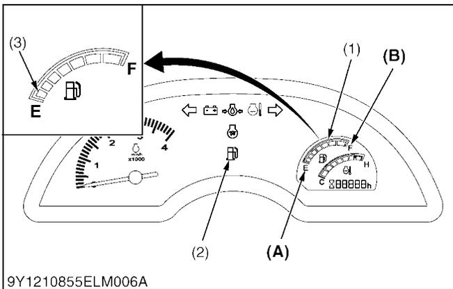
Fuel level gauge and fuel level sensor are connected by the wiring.
