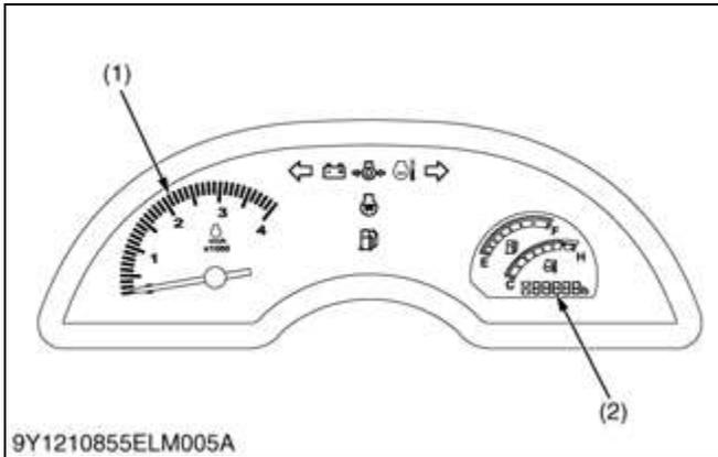
The electrical hour meter and tachometer is equipped on the meter panel.
