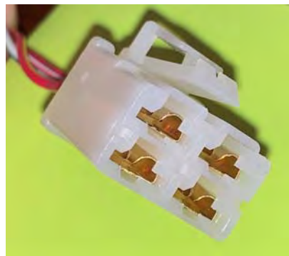
Relay 4-pin connector (Female spade)
