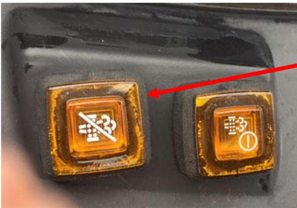
**DPF Inhibit Switch** This switch, if pressed, and if illuminated, prevents the tractor from beginning a regeneration. Under most conditions, you leave it unlit, which is the default when you start the tractor, and which allows automatic regeneration when needed. You might press this inhibit button during operation if you are, for example, working in a dusty, highly flammable environment. The exhaust pipe gets HOT during regeneration!
