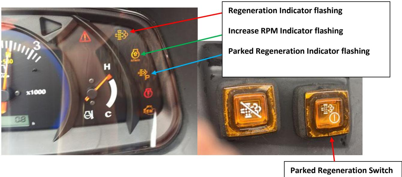
A parked regen requires that you lower implements and turn off PTO if on, set the throttle to idle, the gears to neutral, put the parking brake on, push the **parked regen switch button**, and so forth. The process is outlined on p19.
