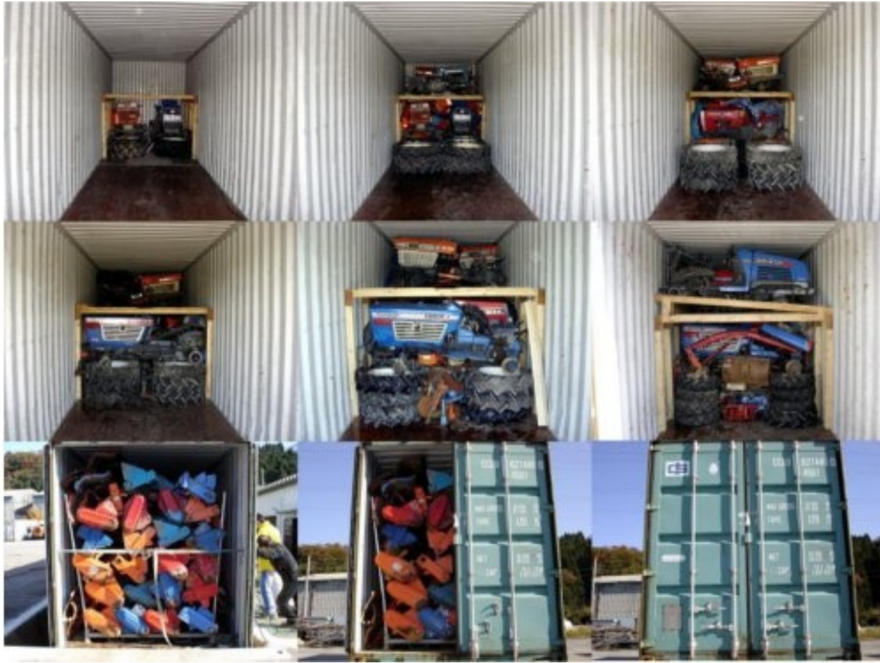
The procedure for loading gray market Kubota, Iseki and Yanmar tractors into shipping containers.
