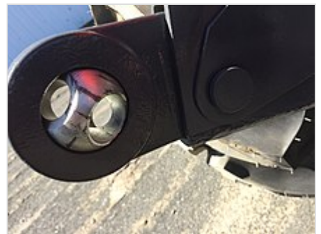
Adjustable three-point ball on lift arm. Ball may be rotated to fit either Category I or Category II implements
