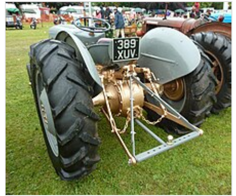
Three-point linkage on a Ferguson 35 tractor.
