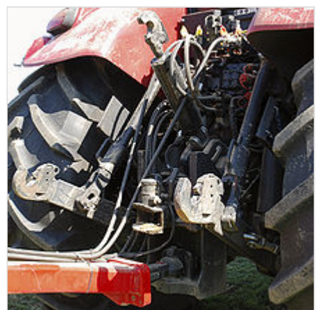
Rear three-point hitch of a Case IH tractor with implement attached by the drawbar
