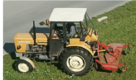
Ursus C-360 tractor and mowing deck, attached by a three-point linkage and driven by a PTO shaft
