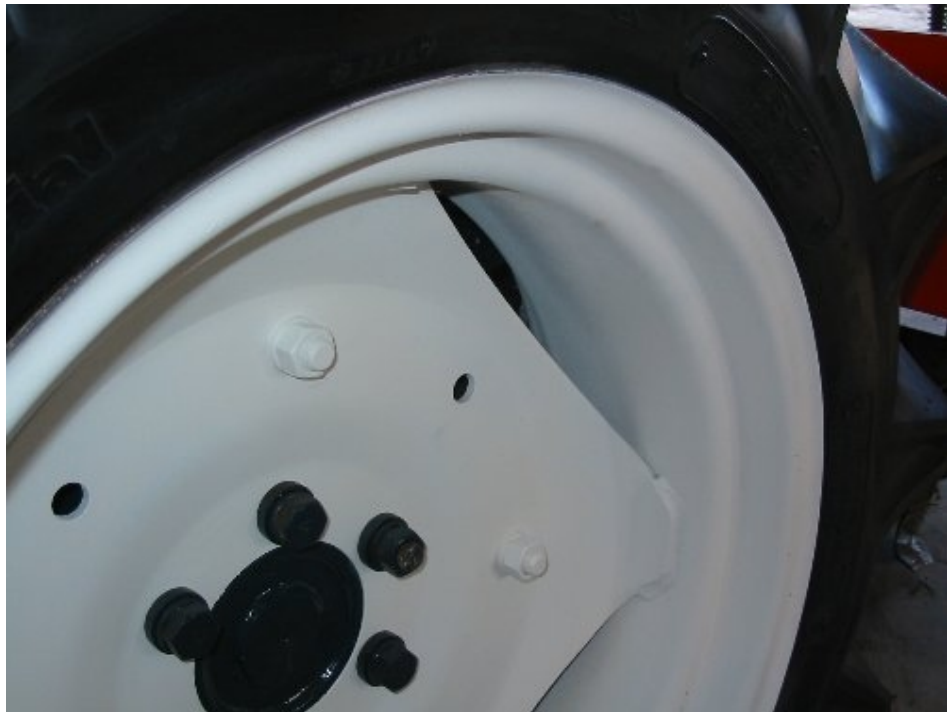
Wheels after prep, masking and painting.
