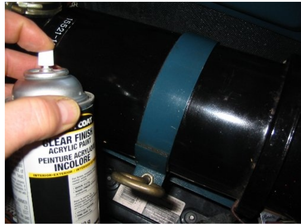
We apply clear coat to the air box, small hoses or compartments in the engine bay - brightens them up like new.
