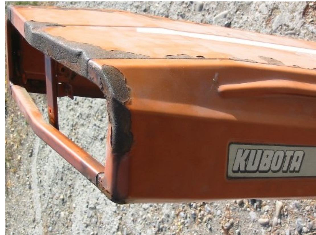
Serious hood rust on the hood of this Kubota is what we are looking to grind down to bare metal with our 60 or 80 grit sandpaper.
