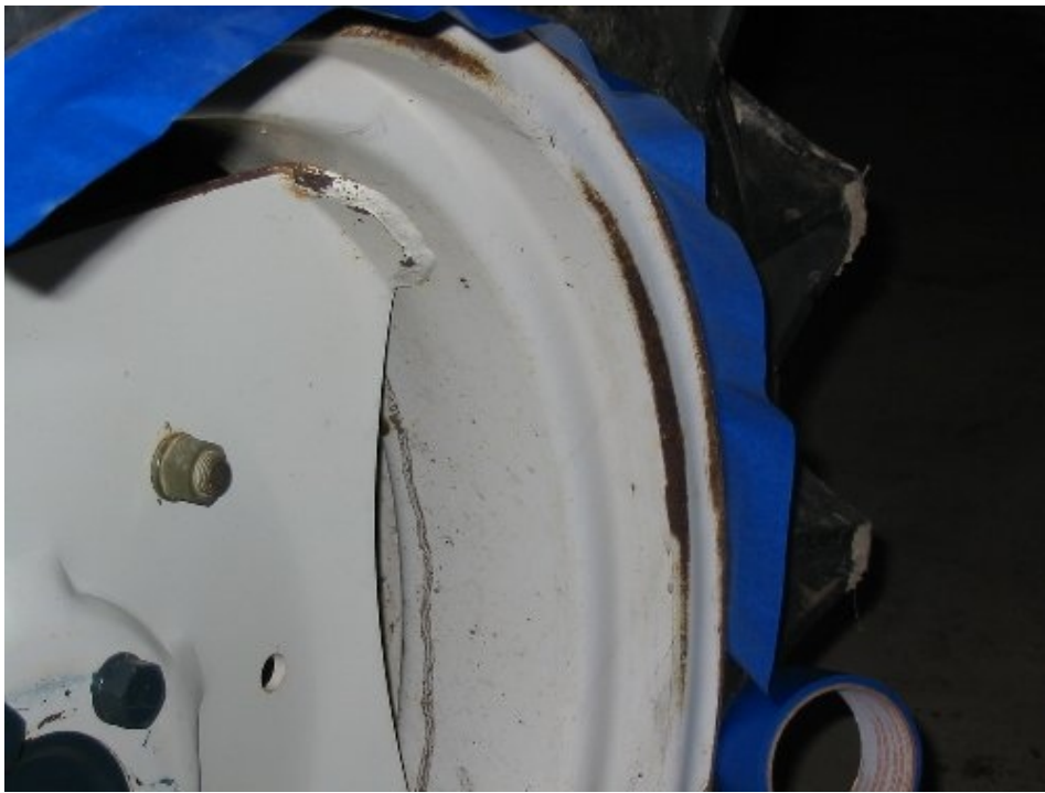
We've used 2" wide tape to mask the wheels on our Kubota.
