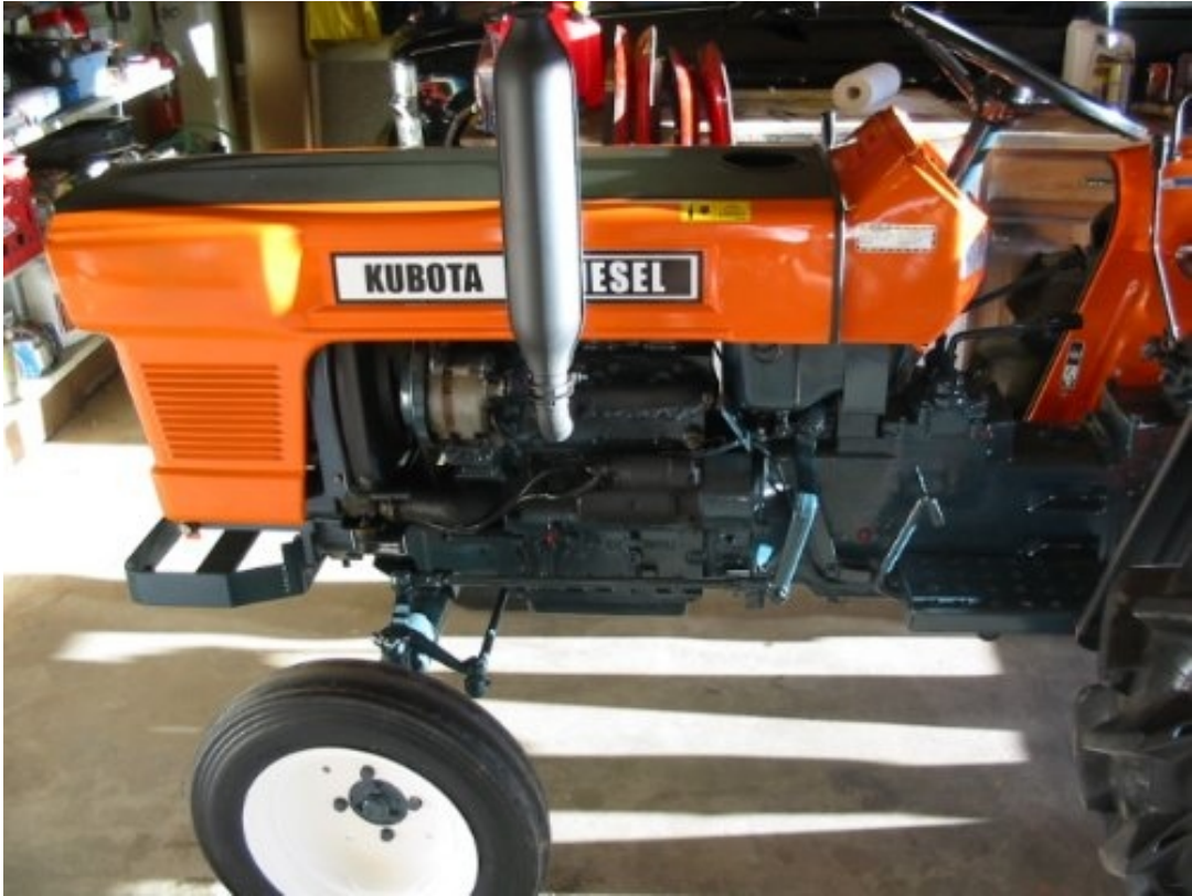
A side shot of the L2000 detailing the painted frame, muffler and stack, wheels and installed decals
