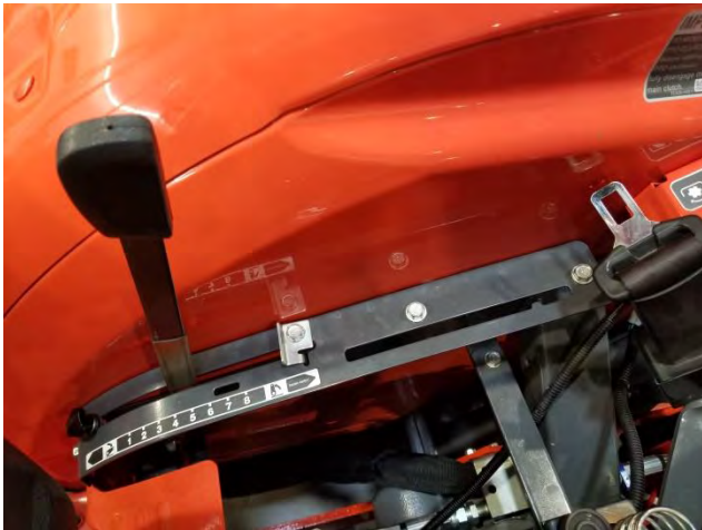
Figure 1: Original lever guide plate for removal
