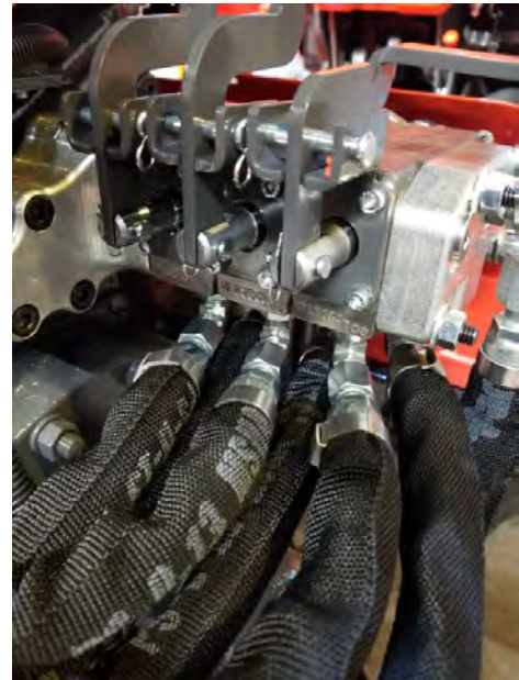
Figure 7: 90 degree fittings installed with approximate 30 degree angle
