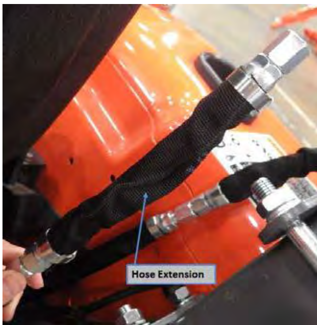
Figure 22: Required hose extensions for backhoe use
