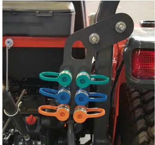
Figure 3: Bulkhead Coupler Mount
