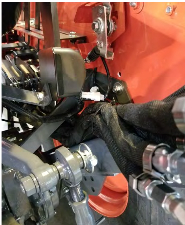
Figure 17: Hose routing for 3PT lift arm clearance
